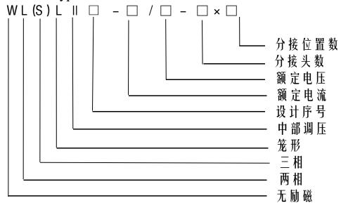
number of tap positions number of tap terminals rated voltage rated current no. design series regulating from middle part Tray-formed three phases two phase no-load regulating
