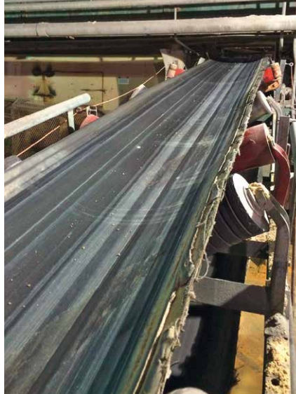
... and after the installation of a pressure roller in combination with a scraper.
