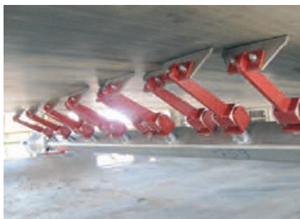
HOSCH scrapers in continuous operation at an open-cast mine
