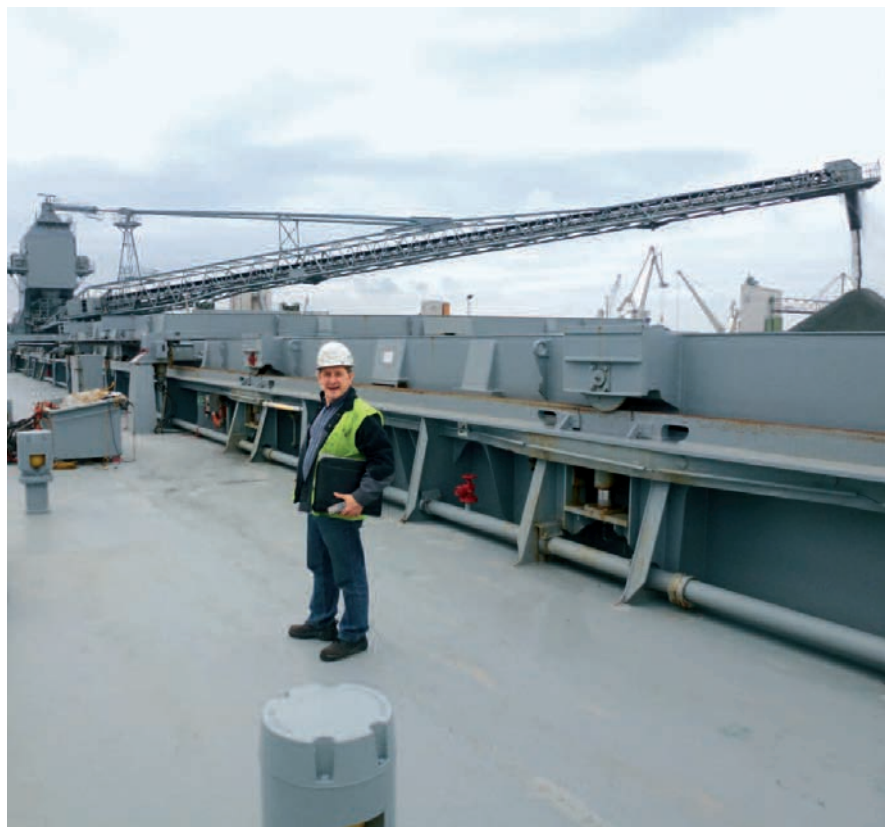
The ship is unloaded with a swivel conveyor. In the foreground: Hubert Kopyto
