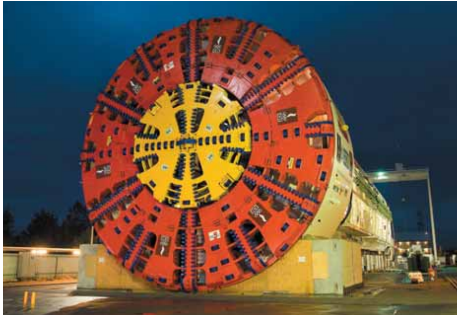
The world's largest tunnel excavator weighs 4,300 tons. It is used together with HOSCH scrapers.
