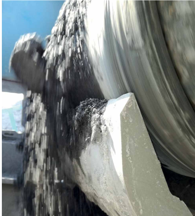
The HD-PU-L prescraper deployed in tunnel construction in South Tyrol.
