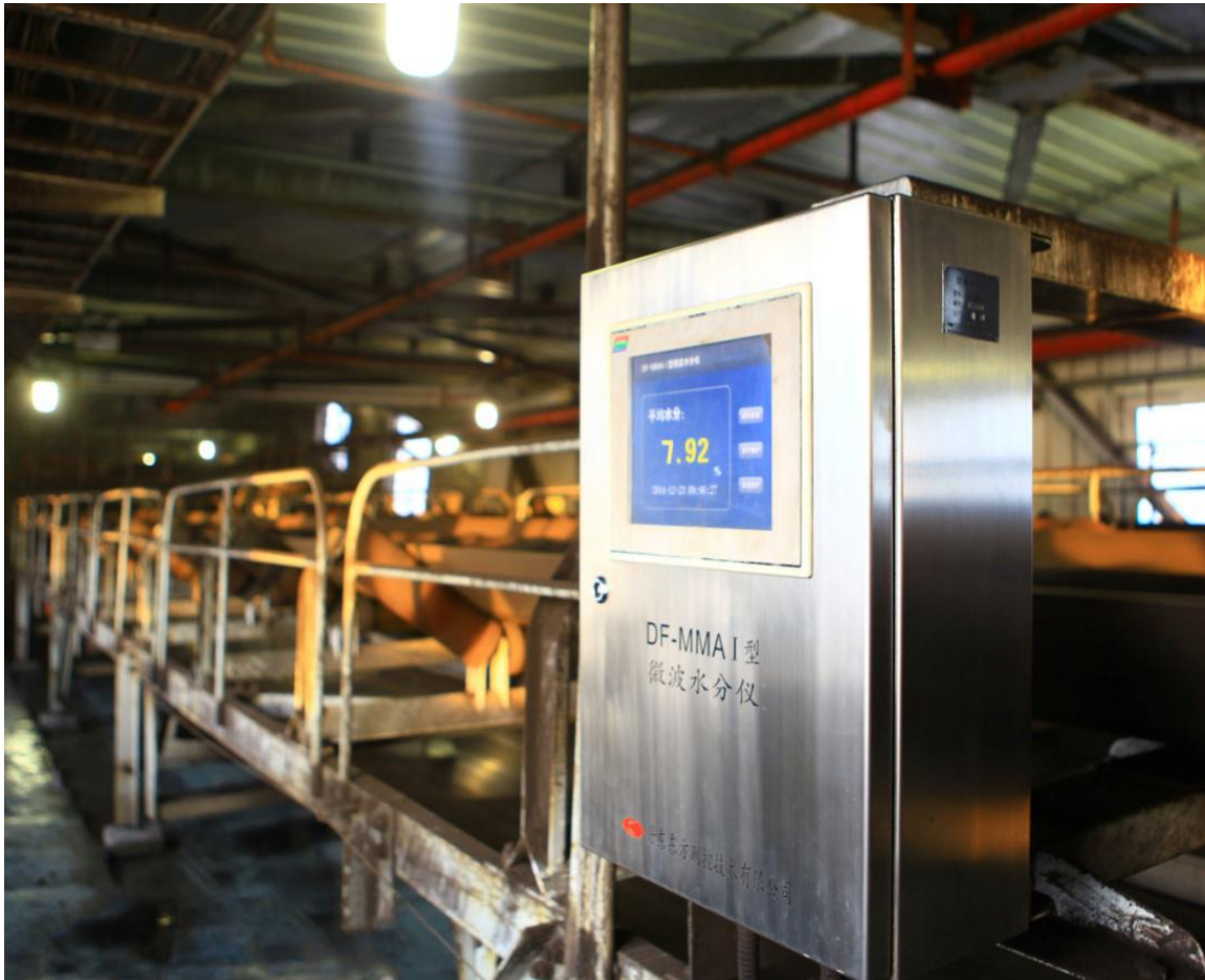
Moisture detection of coal as fired
