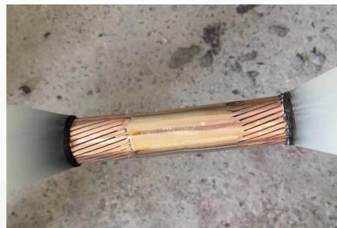
Core fusion splicing
