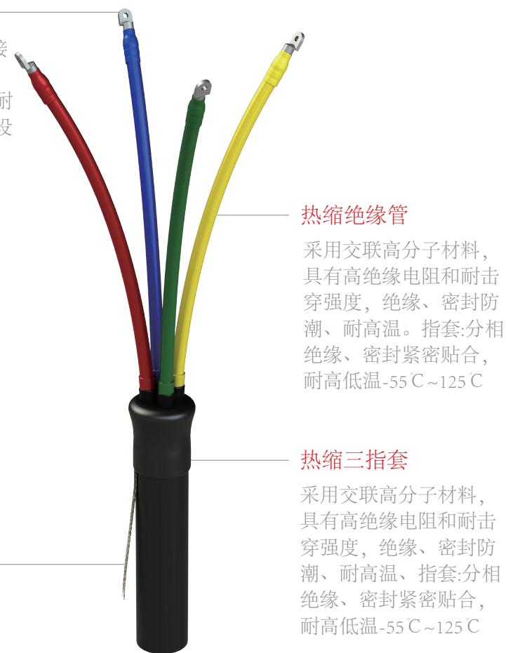
1-3kV热缩终端 1-3kV heat-shrinkable cable termination
