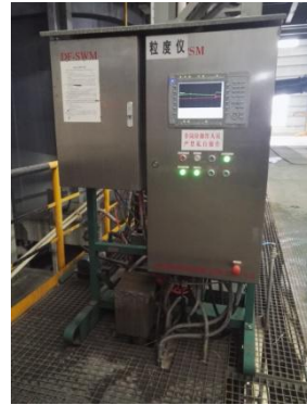
Particle size measurement at cyclone overflow in copper processing plant
